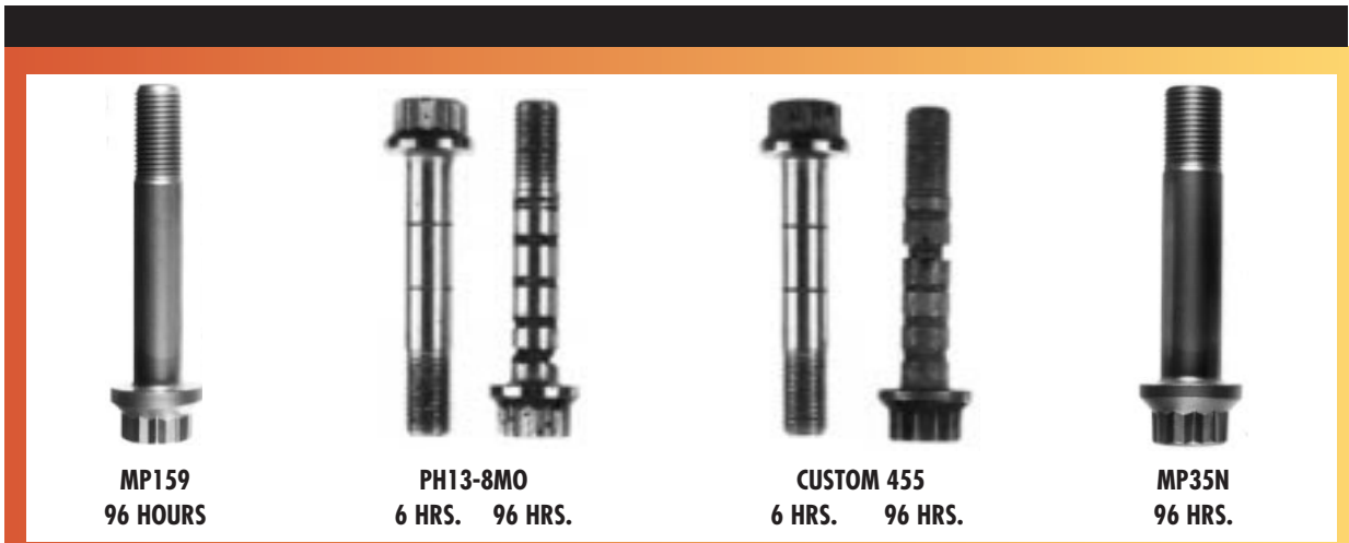
Bolts crevice corrosion tested in 10% ferric chloride solution. The MP35N and MP159 alloy bolts show no visible evidence of attack, in sharp contrast to the other two high strength fastener alloys.
